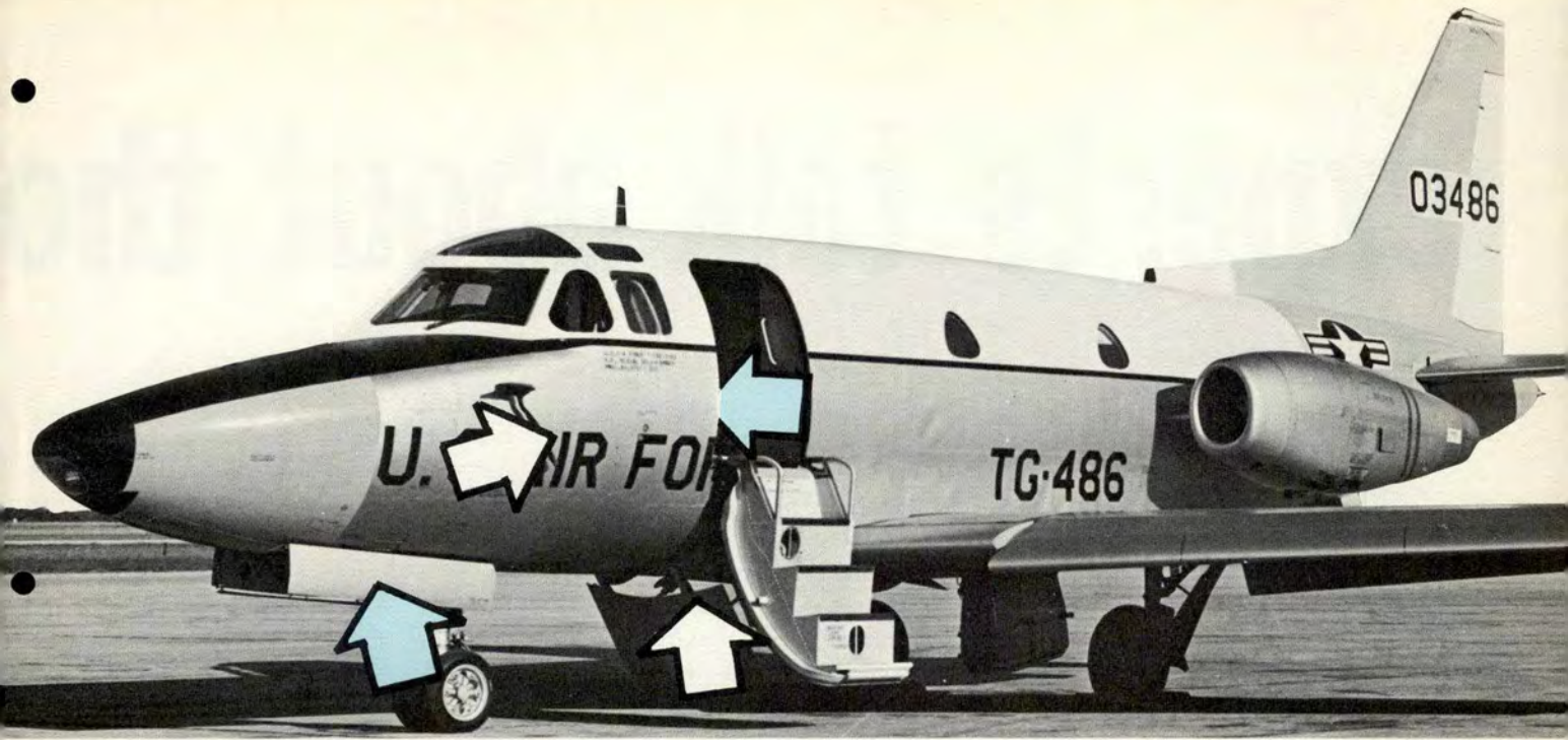
Two drains located one on either side of nose wheel well.
