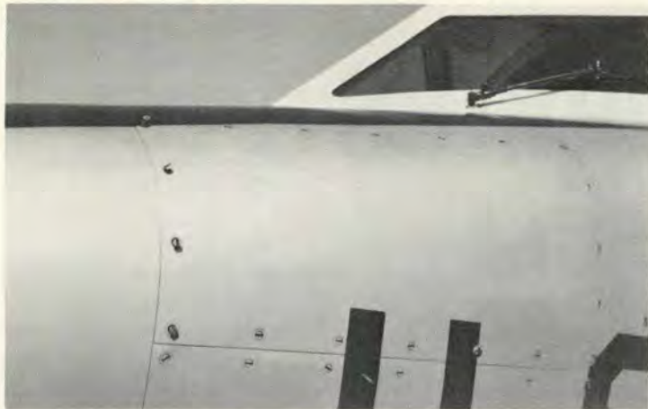
This improperly latched panel would come off in flight.
